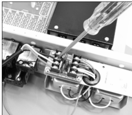
Wire line-voltage connections to the appropriate terminals.
